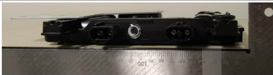
Figure 6: IQ7 Connector side
