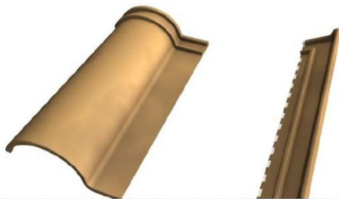
Tiles cutting for left flashing
